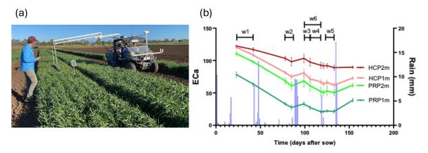
UQ-QAAFI's RootPhenomobile surveying the 2024 wheat trial at Gatton, Qld (a), and (b) readings from the RootPhenomobile showing the decline in soil water during the trial for one plot at different integration depths 0-0.5m (dark green), 0-1m (light green), 0-1.5m (pink) and 0-3m depth (red). In (b) w1 to w6 shows the definition of dry windows during which root traits could be derived.
