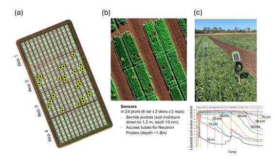
Standard twin plot trial design across all researcher-managed trials for wheat during 2024, and additional continuous soil water monitoring at the Gatton trial using Sentek Drill&Drop sensors on 24 plots including 6 varieties, two plant densities and two replications.
